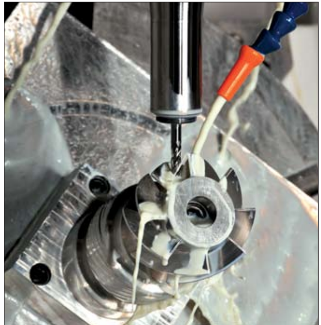
The Okuma machine tools, including the five axis MU-500 seen here, have allowed XL Tool to machine complex parts for new markets.
