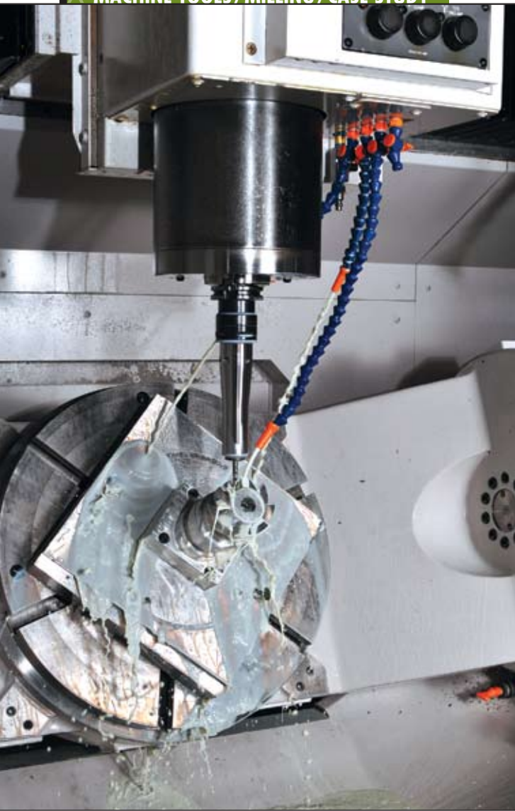
Top: The Okuma MU-500 five axis machine tool in action at XL Tool.
