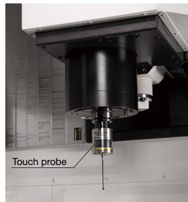
Auto zero offset, auto gauging (radio-controlled touch probe)
