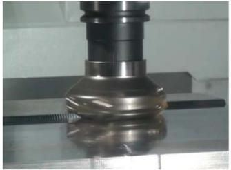
**End milling capacity: 672 cm<sup>3</sup>/min (S45C)**
