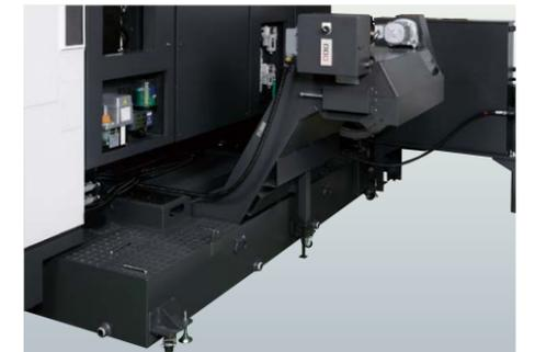
Off-machine chip discharge (lift-up chip conveyor)
