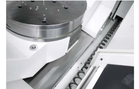
In-machine chip discharge (coil) (Standard)
