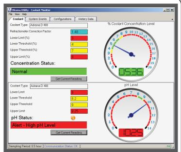
Coolant Concentration and pH Level Status On-screen dashboard gives critical coolant concentration and pH level information right on the THINC-OSP control.
