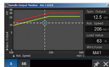
The specified spindle output (red line: short time rating, green line: continuous rating) and the spindle output in current cutting (blue circle) are simultaneously displayed on the screen, for real-time view of power reserve during cutting. This allows speeding up cutting by increasing the spindle speed or feed rate while monitoring the graph to ensure that the blue circle does not cross the lines.
